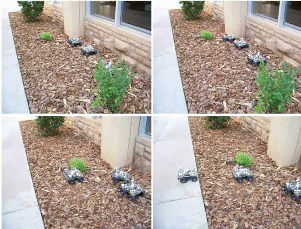
Fig. 19. Three outdoor robots with Physicomimetics and an obstacle avoidance module.
